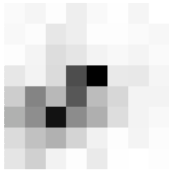
Figure 7: Simulated K-band image for TRICK when guiding on an off-axis star. There are two peaks within the 8 \times 8 pixel region, which presents a problem for a peak finding algorithm.
