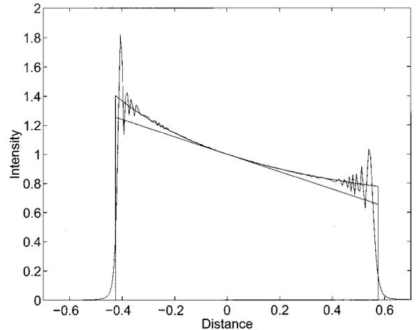
Fig. 3. Comparison of Fresnel (irregular curve), non-linear (smooth curve) and linear (straight line) intensity curves for a cubic aberration. Here  $\lambda = 0.1 \mu\text{m}$ ,  $z = 10 \text{ km}$ , and  $W = 100x^3 \mu\text{m}$ .
