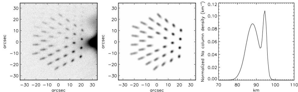
Fig. 1. Images of the LGS on January 26, 2005, formed by adding focus across the primary mirror segments (left), and a corresponding simulated image (center) using an estimated sodium profile (right). The launch telescope is located to the right of the pupil, where the Rayleigh scatter can be seen.
