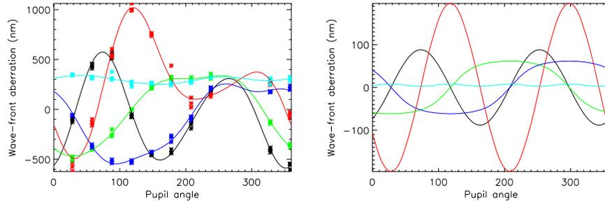
Fig. 2. The measured (left) and modeled (right) LGS aberrations as a function of pupil angle near zenith. The curves are,  $0^\circ$  astigmatism (red),  $45^\circ$  astigmatism (black), spherical aberration (light blue),  $y$ -coma (green) and  $x$ -coma (dark blue).
