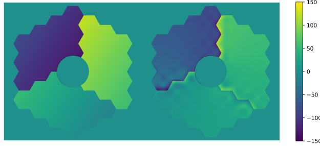
Figure 8: Simulated residual wavefront (nm) when applying 99 nm RMS of segment piston with the adaptive optics loop open (left) and closed (right). No other disturbances are present.
